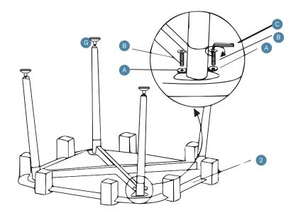
Attach 4 x bolts (E), 4 x spring nuts (F) and 4 x washers (D) to frame (2) as shown. Tighten with an Allen Key (H).
